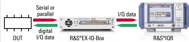
FIG 2 Recording (red) and playing (green) of digital I/Q data. The R&S®EX-IQ-Box converts the I/Q data into the Rohde&Schwarz specific format.
