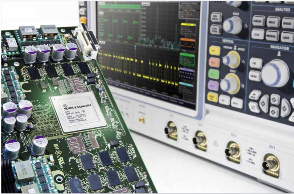
FIG 6 The high-speed ASIC in the R&S®RTO oscilloscopes from Rohde&Schwarz.
