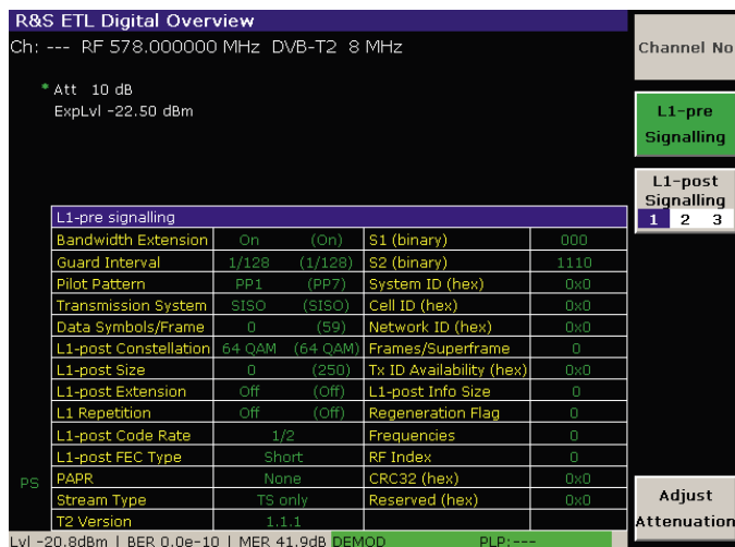
FIG 1 Overview of L1 pre-signaling.
