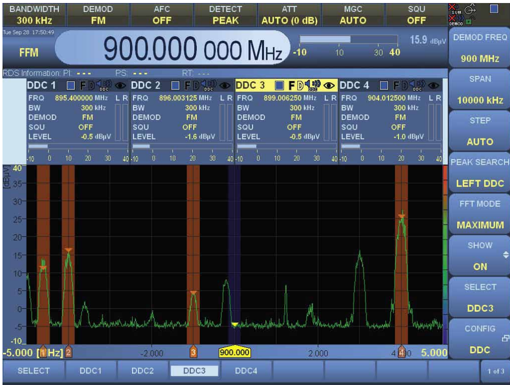
FIG 3 The four digital downconverters provided by the R&S®ESMD in use. Each of the orange-colored bars in the IF panorama indicates the current position and bandwidth of a DDC. Their configuration can be read off from the four status fields above.
