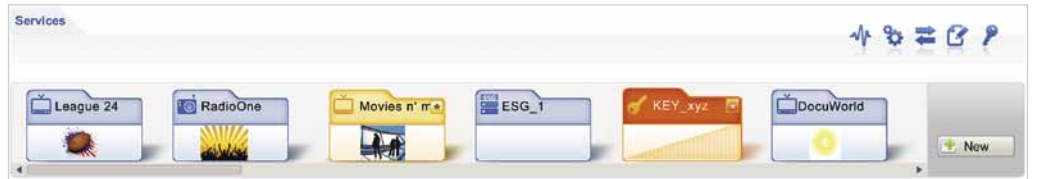
FIG 4 Services slider. The service type is identified by the miniature logo on the upper left. Modified services are highlighted in orange.
