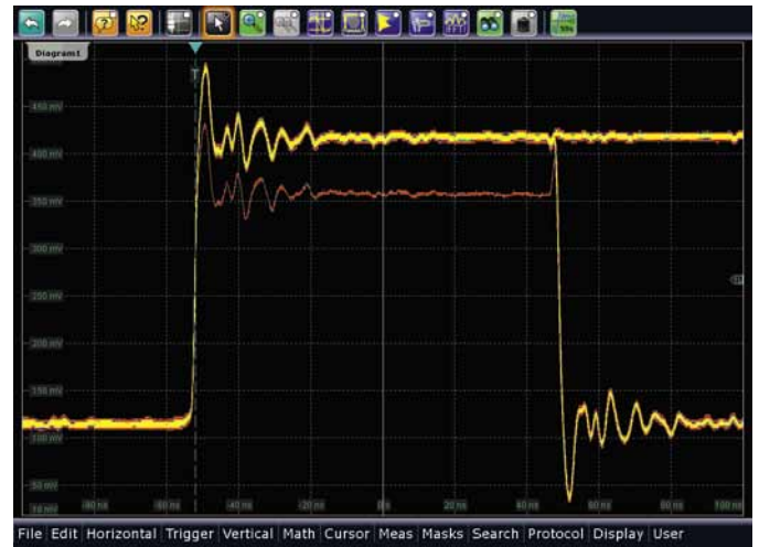
FIG 3 High acquisition rates mean rare signal faults are detected faster. In persistence mode, they are highlighted in color for easy identification.
