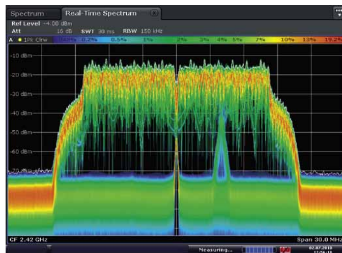
FIG 3 Superposition of a WLAN and Bluetooth® signal in the ISM band. The persistence mode makes it possible to clearly identify the different signals.
