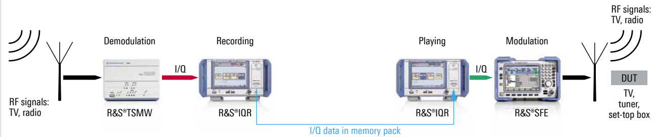
FIG 4 Separate recording and playing of broadcast signals.
